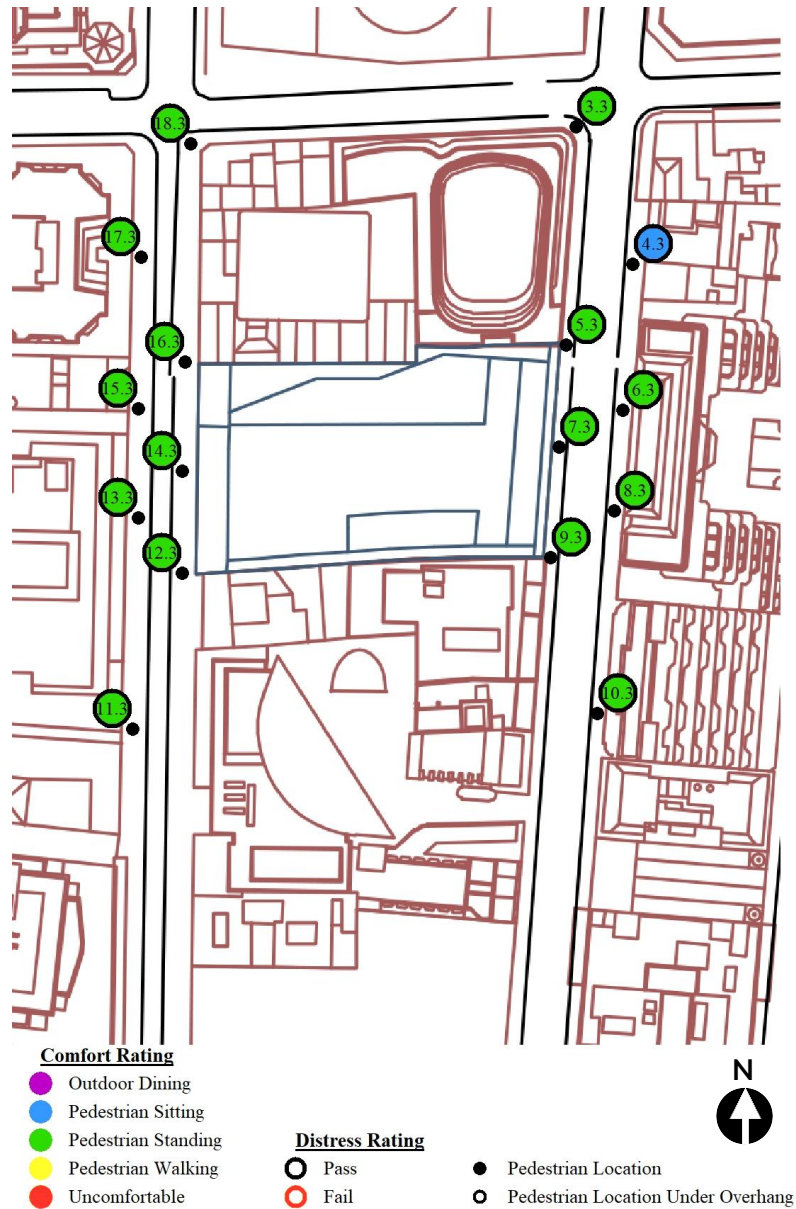
Figure 10: Pedestrian wind speed measurement locations with comfort/safety ratings. Ground – Configuration C: Proposed mixed-use
